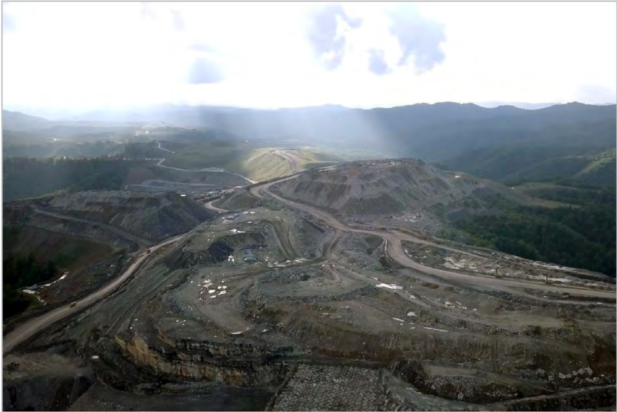
FIGURE 2: MOUNTAINTOP REMOVAL: COAL SURFACE MINING
